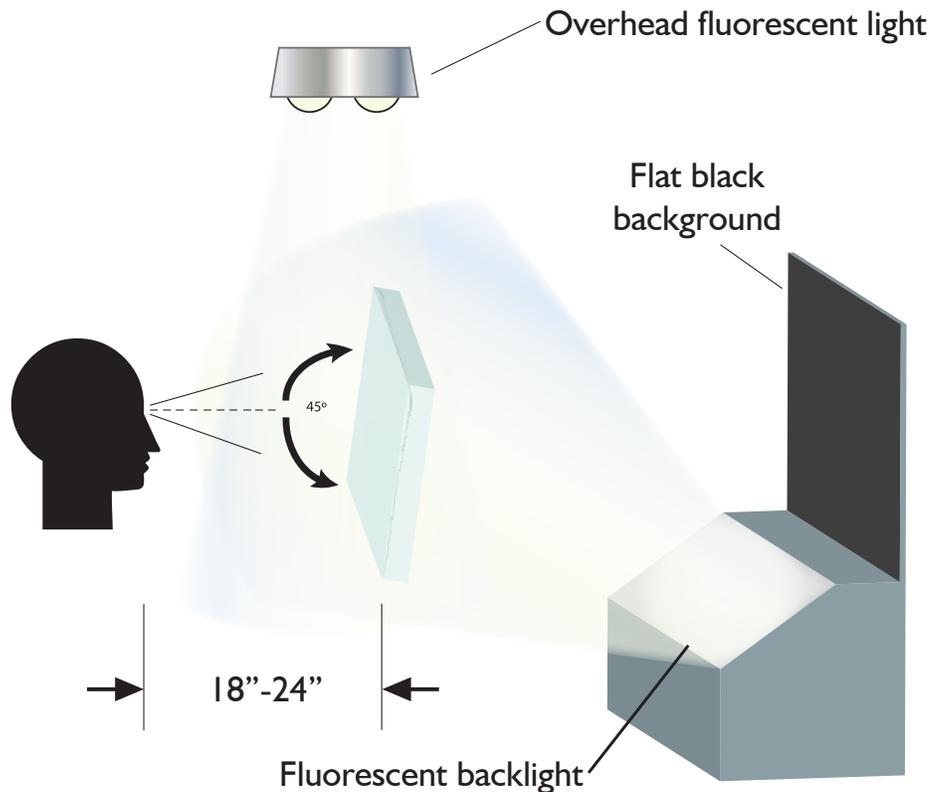
**Note: Inspection Method To Be Used Only When Parts Are Questionable to Standard 80/50 SQC**
