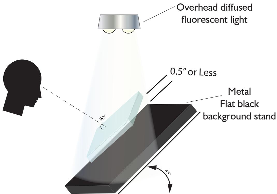
**Note: Inspection Method Starts in Transmission and is Rotated into Reflection**
