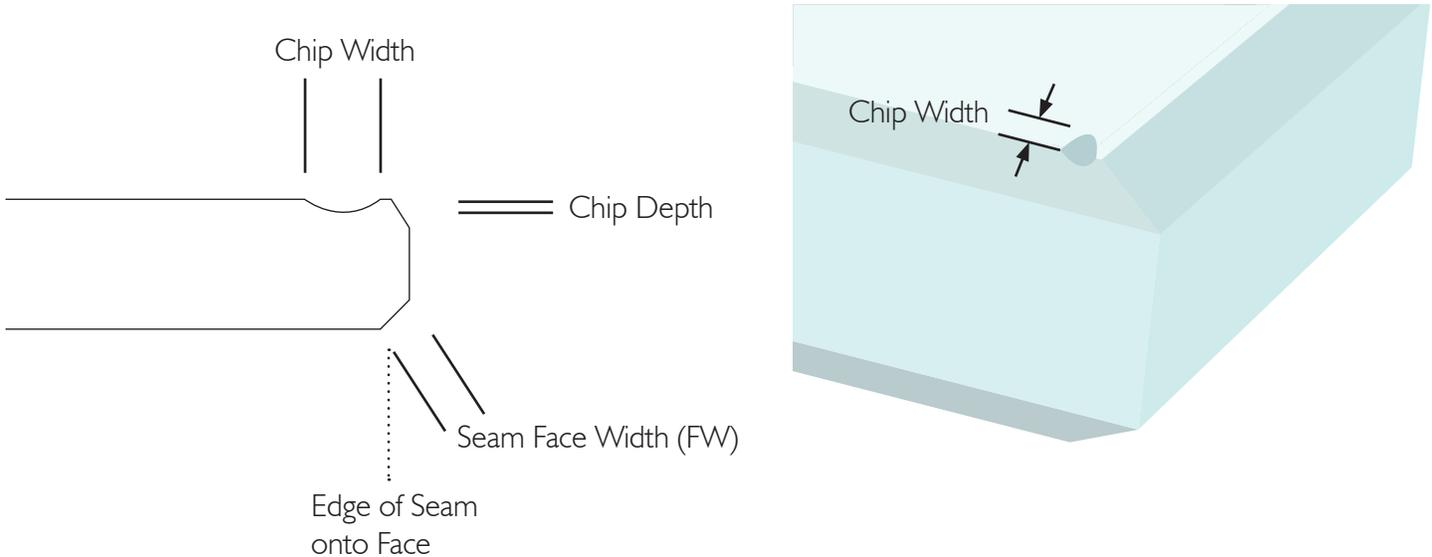
The chip allowance specification will vary by part depending on the glass thickness and processing methods, as well as product application and glass mounting method.
