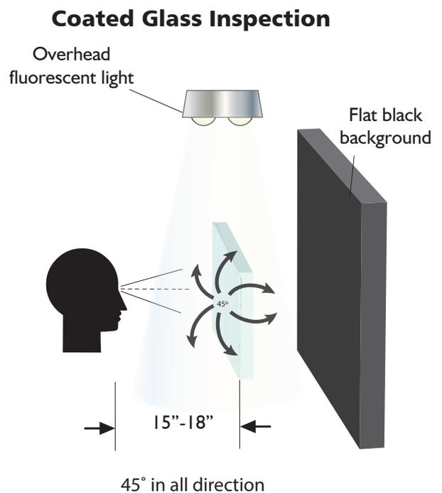
**Note: Inspection Method Starts in Transmission and is Rotated into Reflection**
