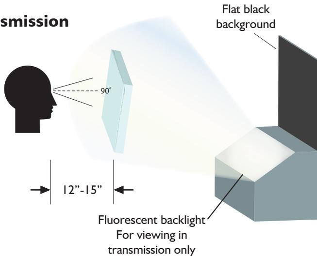
**View perpendicular to the eye, at 12"-15", in transmission for 2-5 seconds against a flat black background and 45° backlight.**
