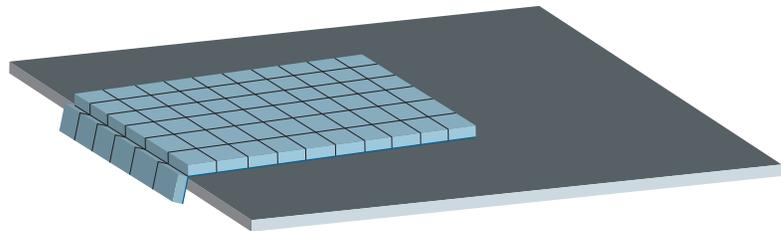
Repeat steps 3 & 4 as needed, being careful not to bend the pattie concave during handling. Store any remaining parts on the vinylized pattie and on a rigid flat surface (as shipped).
