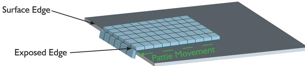
Carefully peel one part at a time from the exposed row. If using a tool for part removal, use bamboo tweezers (these can be purchased online from manufacturer Uxcell; there are several options). **Metal tweezers will chip/scratch/damage glass and should not be used.**
