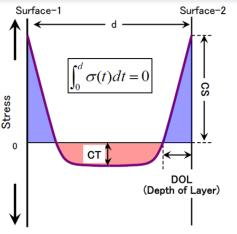
d – Glass Thickness DOL – Depth of Layer CS – Compressive Stress CT – Central Tension CT = (CS\*DOL)/(d-2\*DOL)
